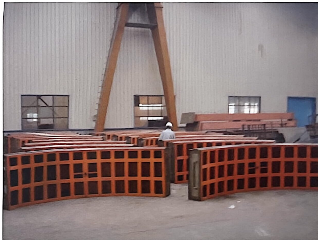
Hangzhou metro steel segment
