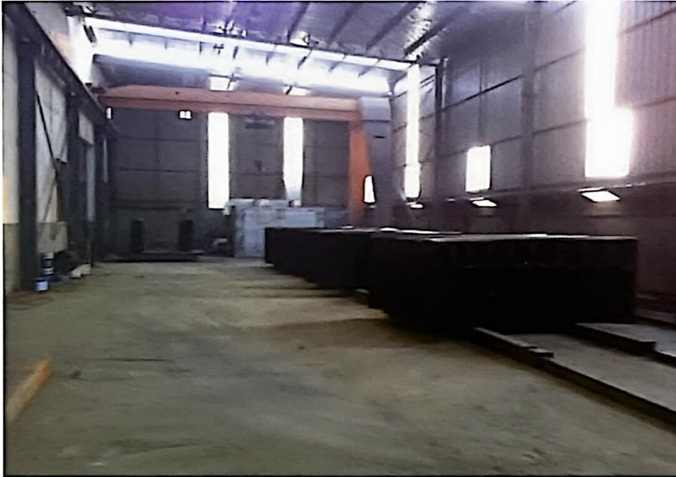
Chengdu metro steel segment
